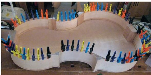
Here's another of those pictures with Bob's technicolor lining clamps on parade, this time on the upper liners. You can see the liners clearly in this picture, and the blocks as well, since they are all made of willow that has a darker color than the maple of the ribs and back. Once the liners are planed to the same level as the ribs and their lower edges beveled and smoothed off, the work on the interior of the body is pretty well done. There'll be some cleanup, I'll put my label in, and then
