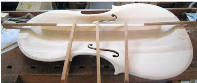
O.K., despite my penchant for truly horrible puns, here's the belly of the bass with the bass bar fitted and glued in. I use simple clothespin-style oak clamps I made myself years ago, which makes the assembly easy to move and which is a great improvement over the heavy steel clamps most of us were taught to use. I find that a lot of string players don't know that this bar is inside the instrument, and those who
