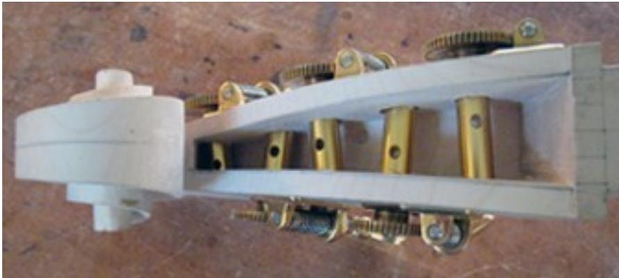
The peg box has been hollowed out, and let me tell you that getting in behind the fifth gear hole isn't an easy task! It was also close on the string hole in the rearmost shaft where the peg box is narrowest, but the string hole is there with just enough room to spare. It is better to fit the tuning machines at this point than it is to attempt it after the pegbox has been
